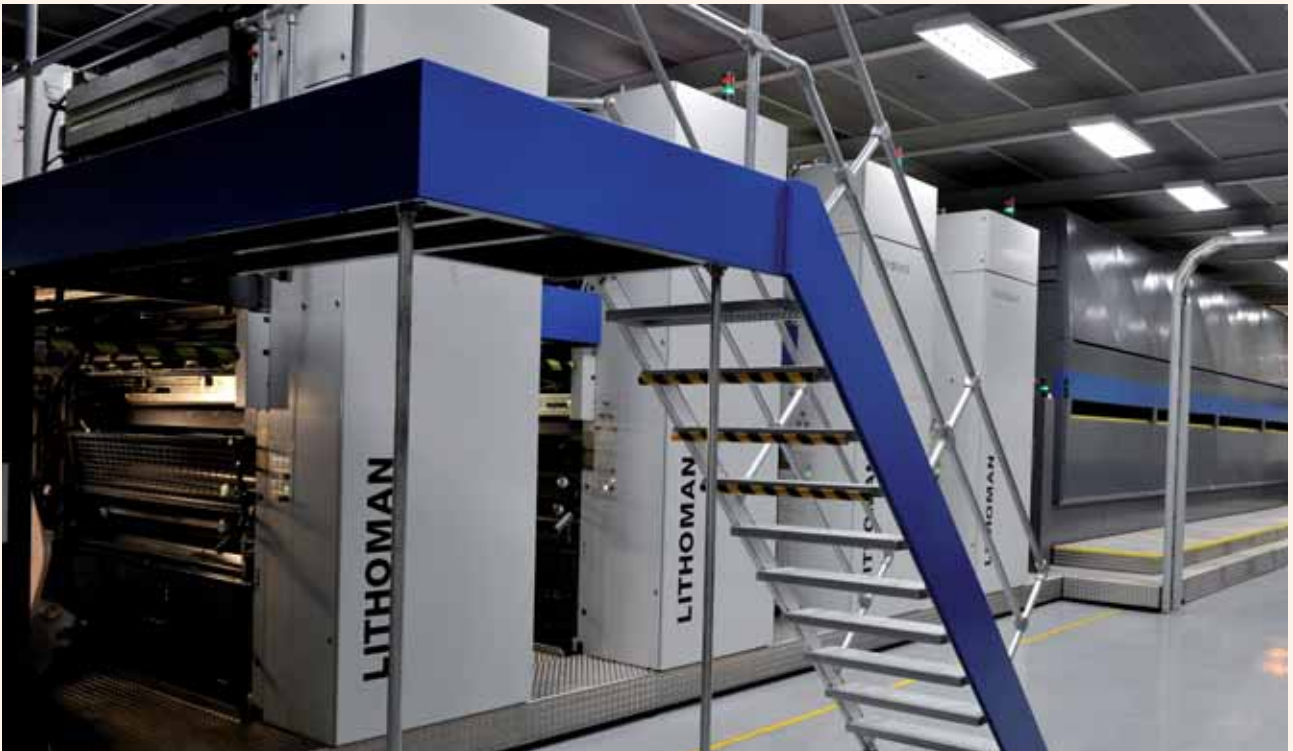
A view of the new Lithoman Web Offset Press installed at CTP Web Printers Isando, Johannesburg during the year
