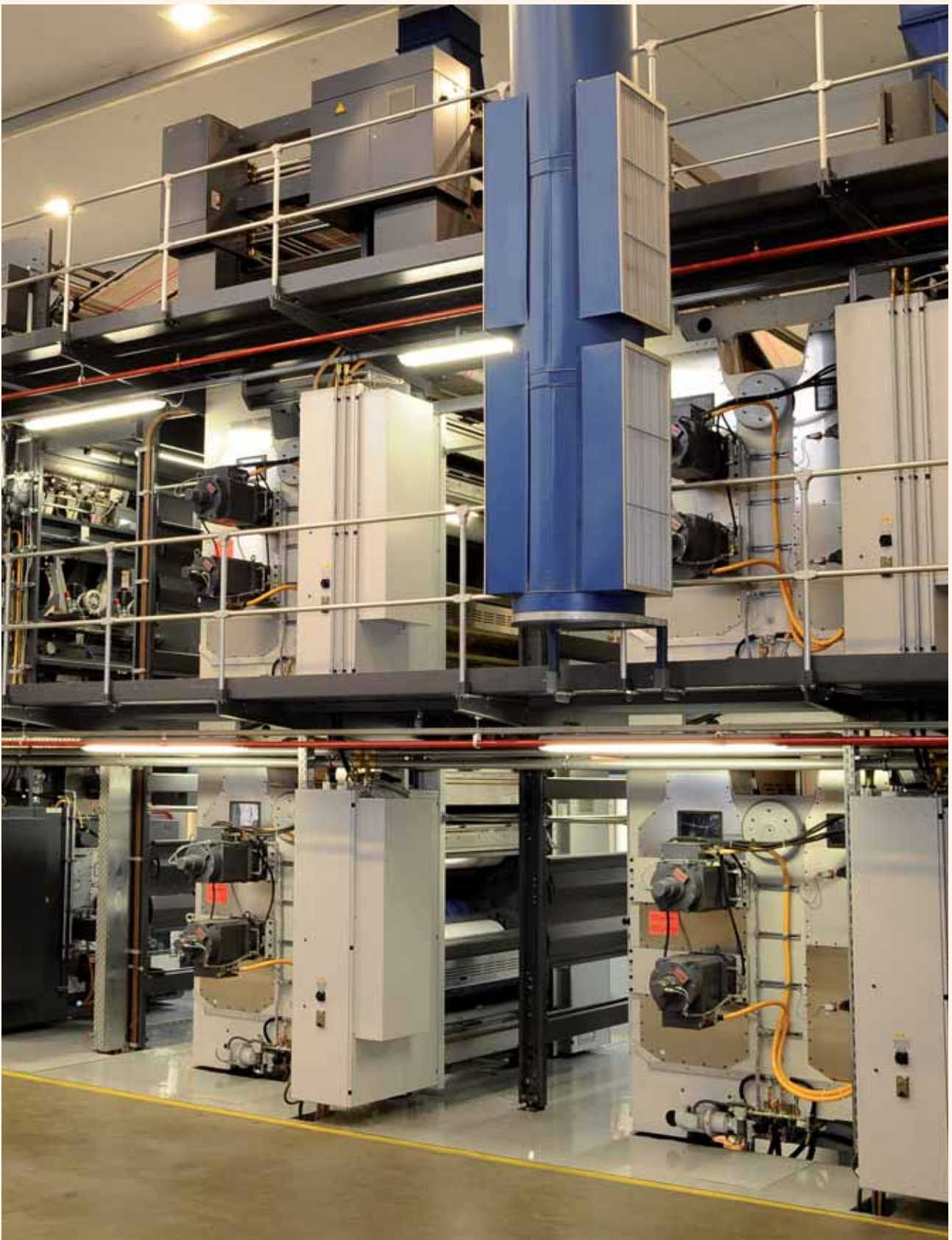
The new Geoman Press built by MAN Roland in Germany and installed and commissioned at the newspaper factory in Industria Johannesburg
