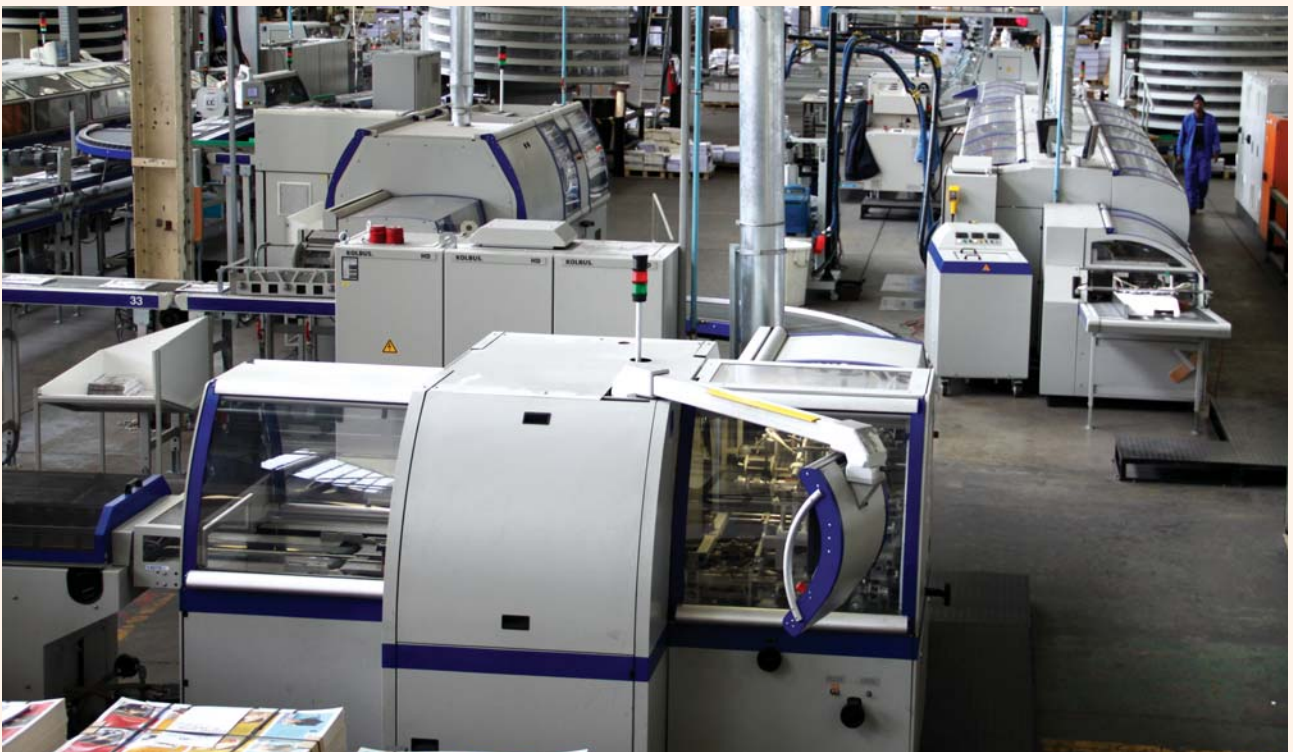
The new Kolbus Publica book binding line which was installed at CTP Printers in Cape Town
